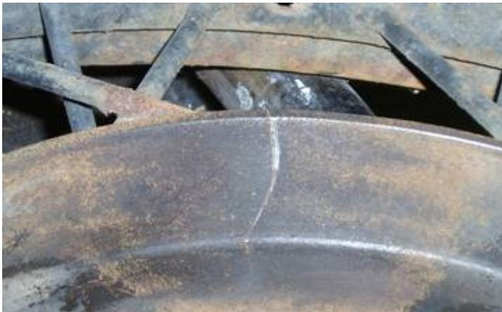
Check for cracks in the hub area.
