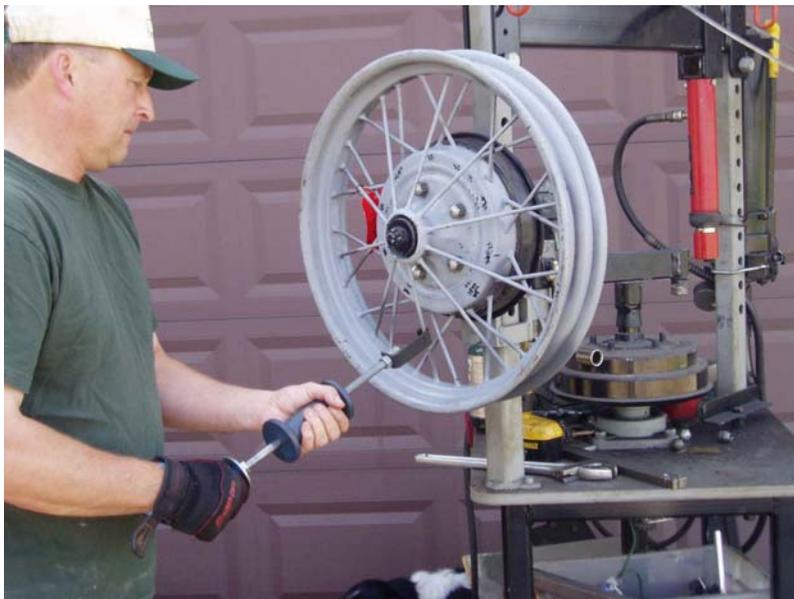
**STRAIGHTEN ALL BENT SPOKES. I AM USING THE SPOKE STRAIGHTENING STATION ON MY HYDRAULIC WHEEL PRESS TO DEMONSTRATE THE PROCESS BUT YOU WILL BE USING THE FRONT AXLE OF YOUR CAR TO COMPLETE MOST OF THE OPERATIONS OF SPOKE STRAIGHTENING.**
