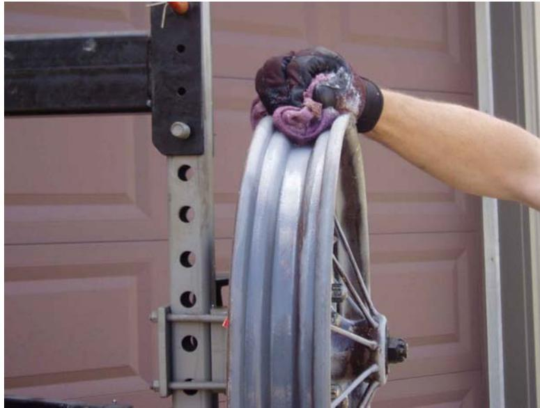
COOL THE OUTER AREA OF THE RIM FIRST BY HOLDING THE WET RAG ON THE AREA PREVIOUSLY HEATED UNTIL THE SIZZLING STOPS AND THEN QUICKLY MOVE TO THE SPOKE AS SHOWN IN THE NEXT PICTURE.
