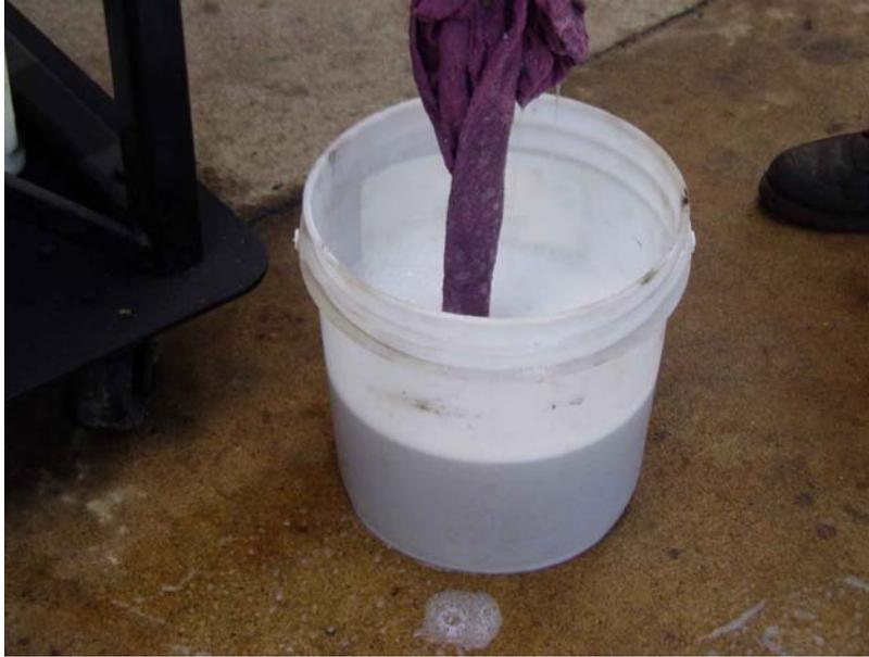
I USE A SOAPY MIXTURE OF COLD WATER TO COOL THE SPOKES. AN OLD SECTION OF A COTTON TOWEL WORKS WELL TO HOLD A LOT OF WATER.
