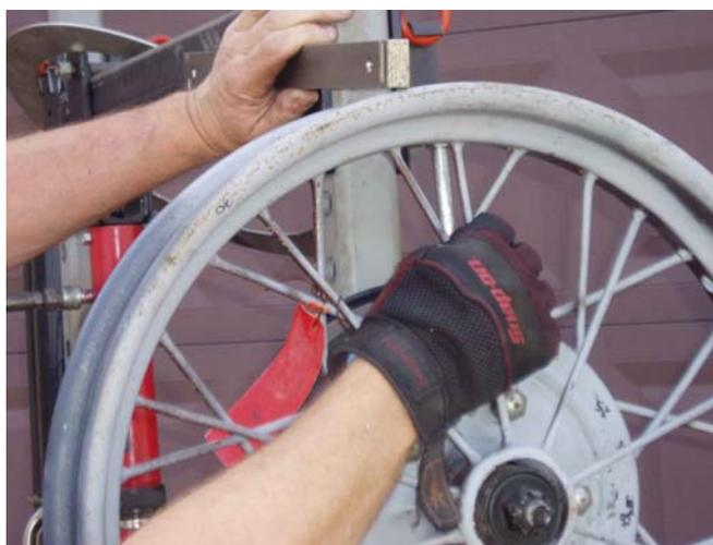
THIS PHOTO SHOWS THE USE OF THE BAR TO ACT AS A GAUGING TOOL TO STUDY THE WOBBLE OF THE WHEEL. ANY THING WILL WORK FOR THIS PURPOSE. (HAMMER HANDLE, LONG SCREWDRIVER, YARD STICK) HOLD THE GAUGING DEVICE AGAINST ANYTHING FIXED NEXT TO THE WHEEL AND SPIN THE WHEEL SLOWLY NOTING THE AREAS THAT NEED TO MOVE "OUT" OR AWAY FROM THE BRAKE DRUM SIDE OF THE WHEEL. SHRINKING THE LONG SPOKES IN THE AREAS THAT NEED TO MOVE OUT WILL PULL THE WHEEL INTO ALIGNMENT.
