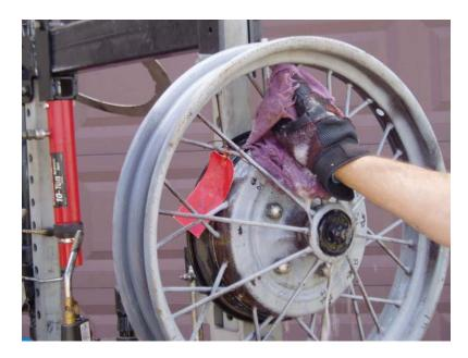
THE RAG IS SURROUNDING THE SPOKE AND QUICKLY MOVED UP AND DOWN THE LENGTH OF THE SPOKE UNTIL THE SPOKE IS COOLED. THE PROCESS IS REPEATED AS OFTEN AS NECESSARY TO PROVIDE THE CORRECTION DESIRED. IT MAY BE NECESSARY TO HEAT TWO OR THREE CONSECUTIVE SPOKES TO ACHIEVE A LARGE AREA CORECTION. THE PROCESS IS THE SAME FOR ALL YEARS OF MODEL A WHEELS.
