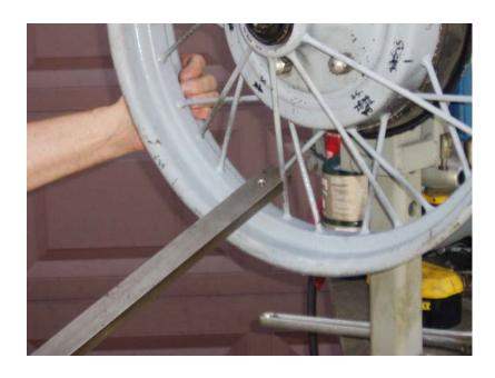
THIS TOOL IS MADE FROM BAR STOCK. IT IS USED TO STRAIGHTEN SHARP BENDS IN THE SPOKES. YOU CAN ALSO USE A CRESENT WRENCH WITH A LARGE SCREWDRIVER THROUGH THE HOLE IN THE HANDLE TO TWIST THE WRENCH.
