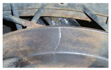
Check for cracks in the hub area.
