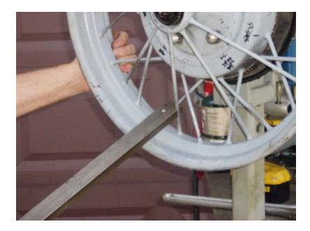
THIS TOOL IS MADE FROM BAR STOCK. IT IS USED TO STRAIGHTEN SHARP BENDS IN THE SPOKES. YOU CAN ALSO USE A CRESENT WRENCH WITH A LARGE SCREWDRIVER THROUGH THE HOLE IN THE HANDLE TO TWIST THE WRENCH.
