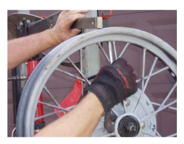
THIS PHOTO SHOWS THE USE OF THE BAR TO ACT AS A GAUGING TOOL TO STUDY THE WOBBLE OF THE WHEEL. ANY THING WILL WORK FOR THIS PURPOSE. (HAMMER HANDLE, LONG SCREWDRIVER, YARD STICK) HOLD THE GAUGING DEVICE AGAINST ANYTHING FIXED NEXT TO THE WHEEL AND SPIN THE WHEEL SLOWLY NOTING THE AREAS THAT NEED TO MOVE "OUT" OR AWAY FROM THE BRAKE DRUM SIDE OF THE WHEEL. SHRINKING THE LONG SPOKES IN THE AREAS THAT NEED TO MOVE OUT WILL PULL THE WHEEL INTO ALIGHNMENT.
