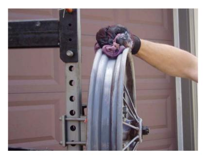
COOL THE OUTER AREA OF THE RIM FIRST BY HOLDING THE WET RAG ON THE AREA PREVIOUSLY HEATED UNTIL THE SIZZLING STOPS AND THEN MOVE TO THE SPOKE AS SHOWN IN THE NEXT PICTURE.
