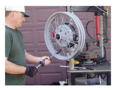
STRAIGHTEN ALL BENT SPOKES. I AM USING THE SPOKE STRAIGHTENING STATION ON MY HYDRAULIC WHEEL PRESS TO DEMONSTRATE THE PROCESS BUT YOU WILL BE USING THE FRONT AXLE OF YOUR CAR TO COMPLETE MOST OF THE OPERATIONS OF SPOKE STRAIGHTENING. (The photo above was staged for the development of this document. Note that safety glasses are missing and should be worn.)
