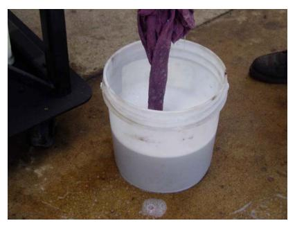
I USE A MILD SOAPY MIXTURE OF COLD WATER TO COOL THE SPOKES. AN OLD SECTION OF A COTTON TOWEL WORKS WELL TO HOLD A LOT OF WATER.
