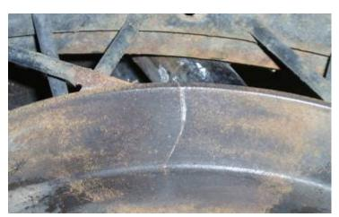
Check for cracks in the hub area.
