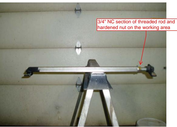
I remove or install about one engine each month and find this spreader saves me a lot of frustration when installing the fresh engine. Most of the time I am working alone and the extra clearance between the rear engine mounts allows the engine to slip right in.
