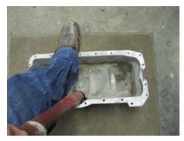
Place one foot on the edge of the pan opposite of the oil pump opening and give it a quick push. The pan will rotate and the dipper tray will pop out. No cuts or bruises...but maybe a little oil on your shoe or pant leg. Works every time!
