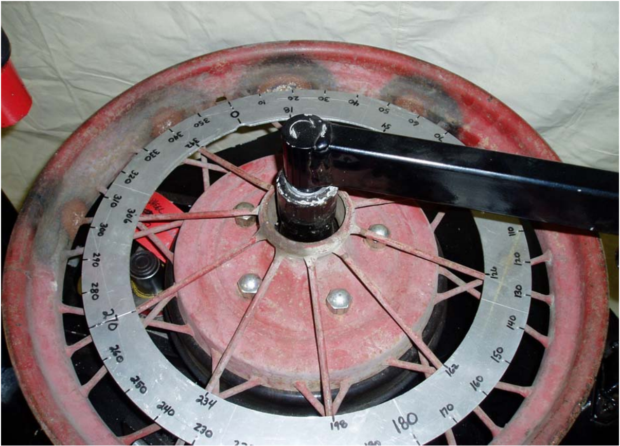
Indexing ring placed on a 21" wheel.
